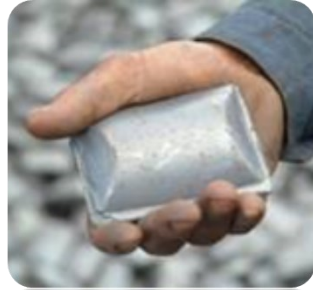
Hot Briquetted Iron
